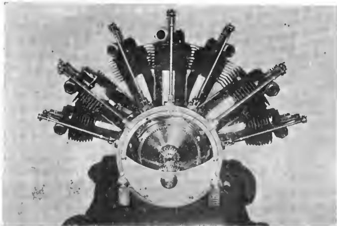
PELTERIE'S SEVEN-CYLINDER MOTOR, SHOWING CAM MECHANISM.
